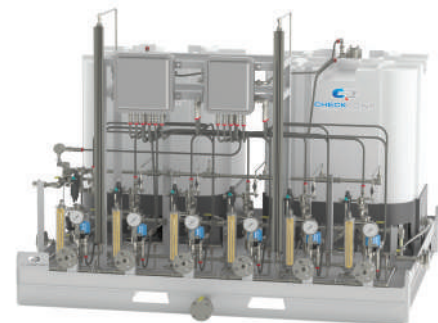
Six pump 1250 injection package with two 275 gallon poly tanks with level transmitters, flow switches and emergency shutdown solenoid valves. Final destination: Bolivia
