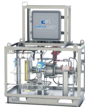
IntellijECT PLC controlled fully automated portable 8400 high pressure injection package with local, remote and automated flow control with flow, pressure and temperature transmitters, actuated discharge ball valve and fire fuse for emergency shutdown. Class 1, Div 1. Final destination: GOM
