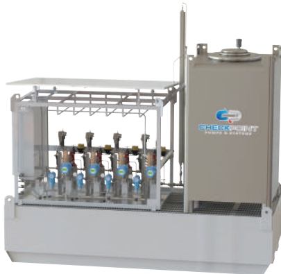
Quad pump pneumatic 1250 auto ready injection package remote and local flow control, solenoid valves for emergency shutdown, flow and pressure transmitters, and 550 gallon 316SS tank with level transmitter and 130% containment bund. Three primary pumps, one fully redundant backup (3A + 1B). Final destination: Marshall County, WV
