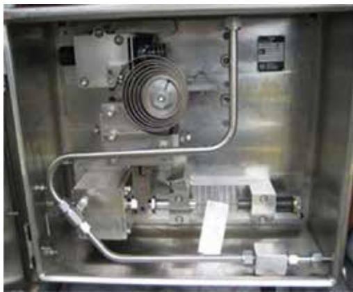
BPIV Buckling Pin Mechanism (Closed Position)
